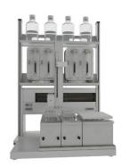
Solid phase extraction (SPE) is a highly selective clean-up technique that eliminates matrix effects and concentrates compounds present as traces to improve analytical detection.
